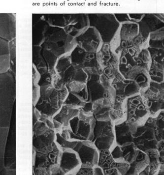
Another example of intergranular cracking but one which shows the effect of heavy oxidation. Magnification is 300X.
